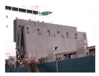
dimensioned for container cargo up to 90 ts per stack.
